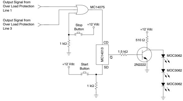
**Diagram 3** shows the main electronic control circuit for controlling the start and stop of the motor each time it is needed. If the start button is pushed on, the Flip Flop (MC14013) is activated triggering the transistor (2N2222) which turns on the optocoupler's LED's which in turn the three triacs (BTA08–600CW) get triggered and finally starts the motor. The motor will stop to operate, whenever
