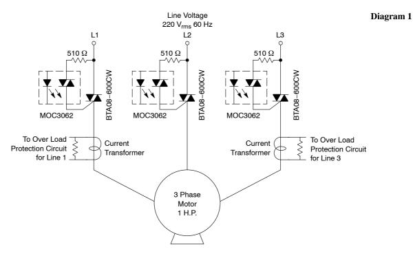
**Diagram 1** shows how three triacs BTA08–600CW3G or BTB08–600CW3G (Ref: BTA08–600CW) substitute the mechanical contacts of the conventional magnetic starter (shown previously) for supplying the power to the three phase 1HP motor once the triacs are triggered.
