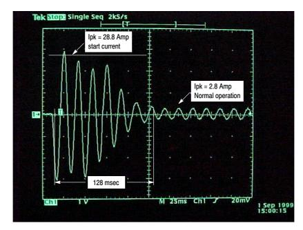
This other plot shows the motor's start current waveform of the three phases when the motor start to operate under normal operation conditions and without mechanical load.
